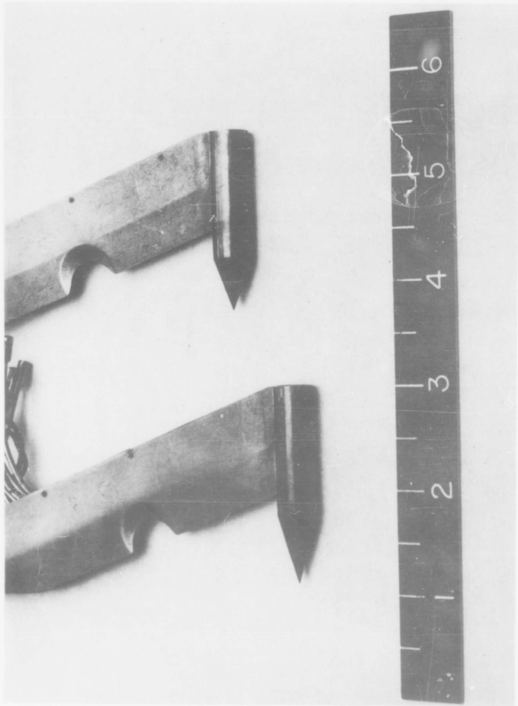
Figure 4. 15-degree (left) and 20-degree (right) semivertex angle cone models
