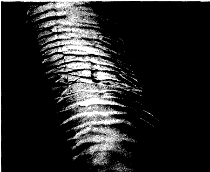
Figure 17. Slip Lines in an Area Near the Fracture Area in Platinum 375X
