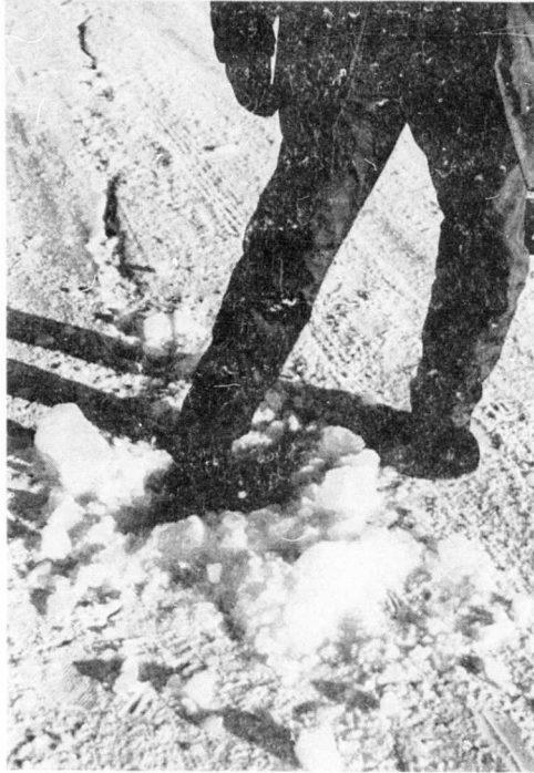
FIG. 8.5 Block of ice lifted from crack and broken by overnight "working" of ice
