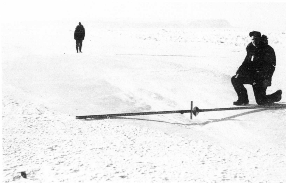
FIG. 6.8. Extent and depth of melt area behind outboard engine of B-47; view west
