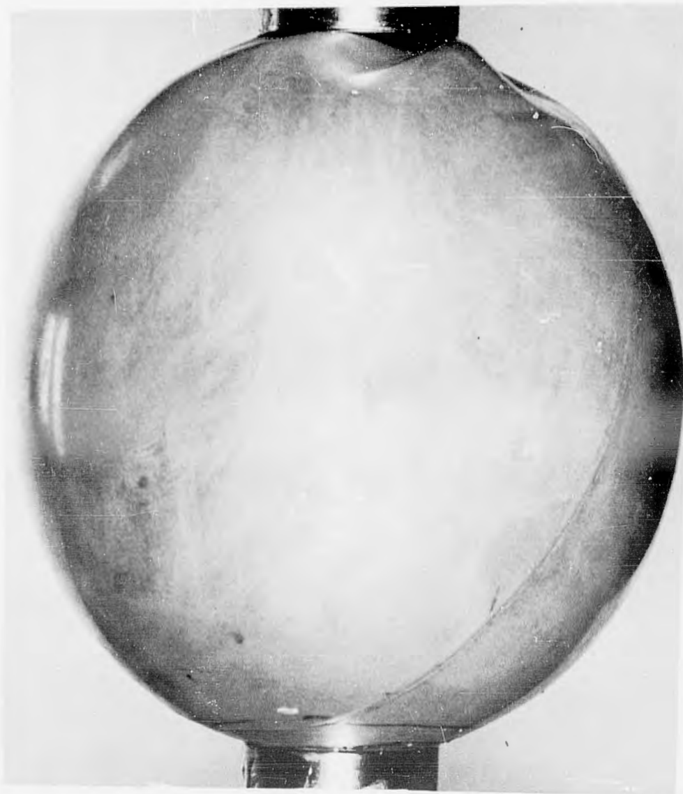
Figure 4. Actual test photograph of a spherical shell in local buckling under twisting torques.
