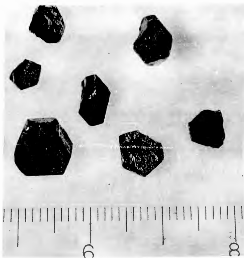
Figure 4. (Zn)Y Crystals. Scale in inches
