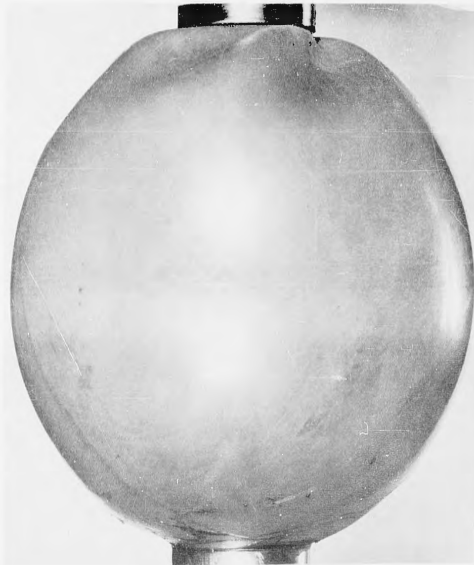
Figure 3. Actual test photograph of a spherical shell in local buckling under twisting torques.
