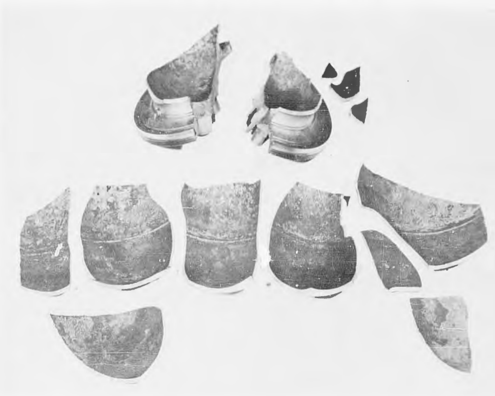
FIGURE 8: H-11 BURST-TESTED VESSEL
