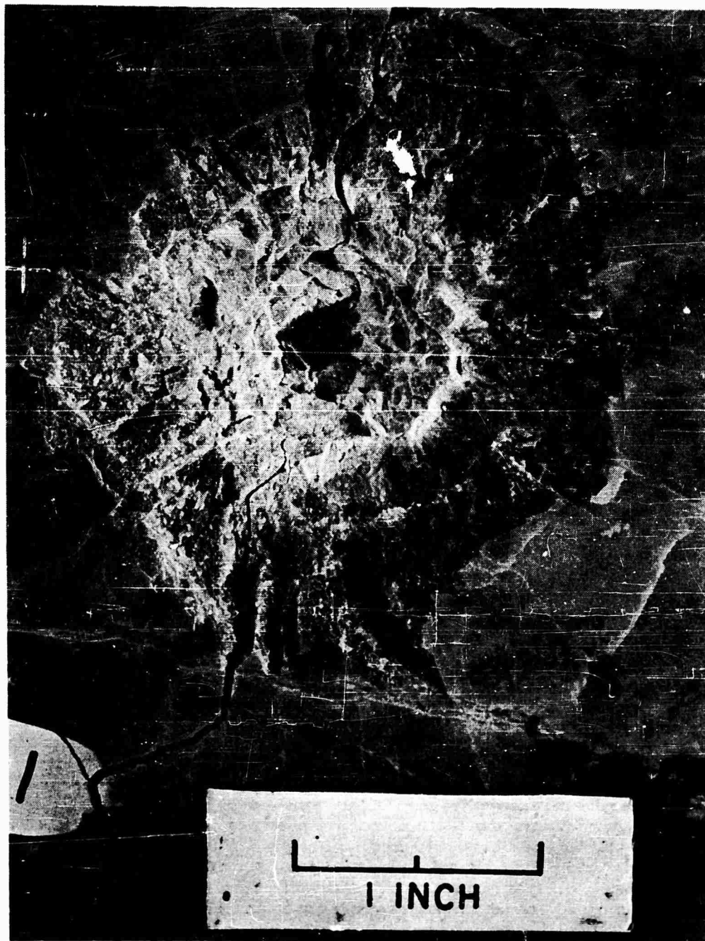
Figure 4. Photograph of Crater Formed in Nephrite by Impact of 0.300 g Cooper-Faced Cylinder at 4.85 km/sec.
