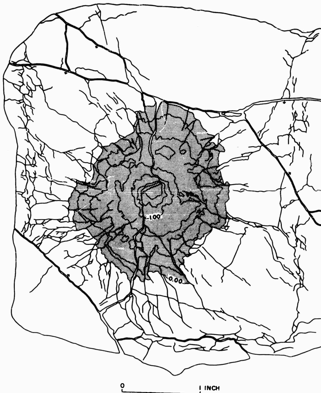
Figure 8. Topographic and structural map of crater in nephrite (see figure 4) showing radial fractures and spall fractures parallel with the sides of the target block. Crater area is shaded; contour interval is 0.25 centimeter.
