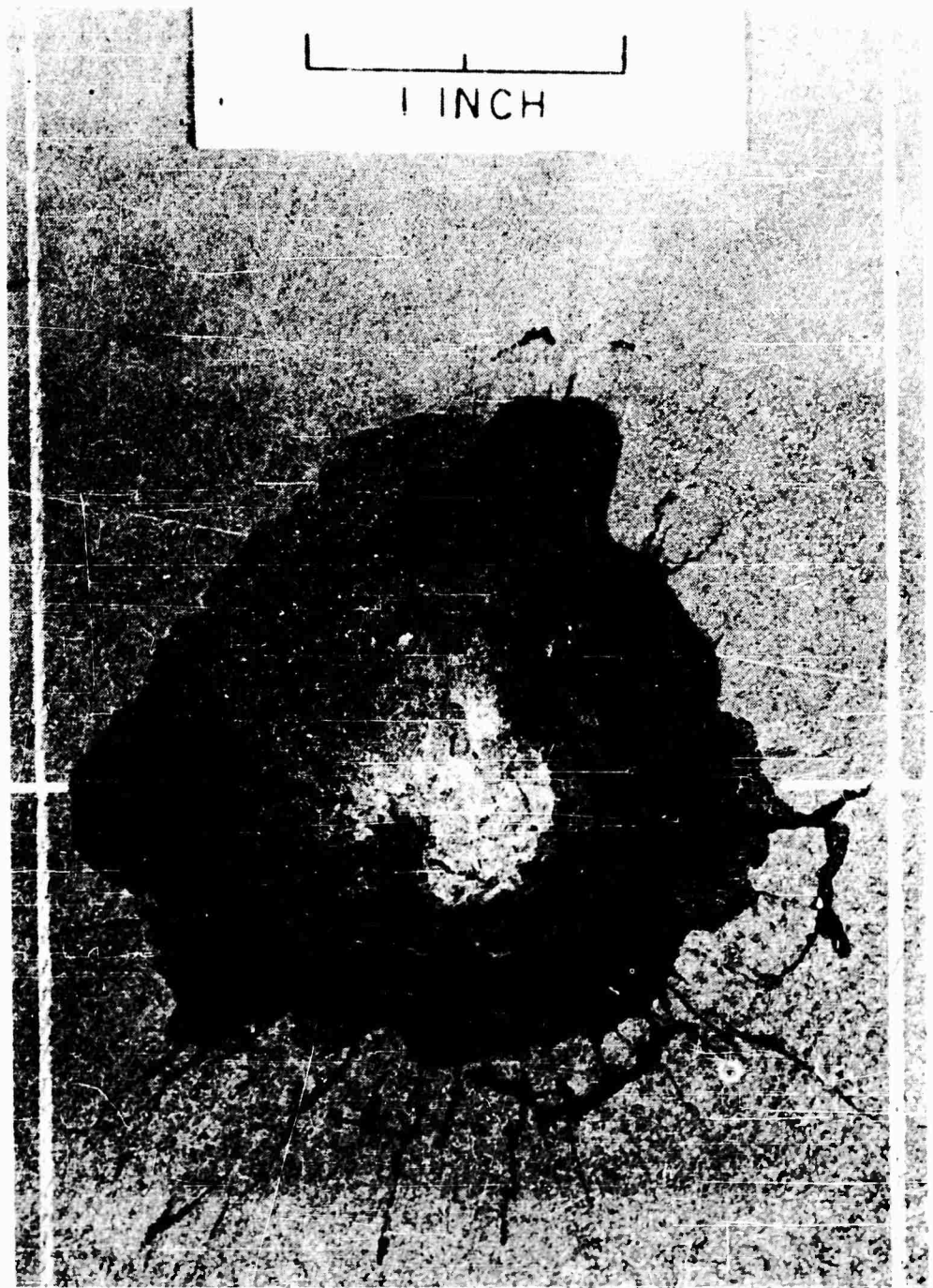
Figure 7. Photograph of Crater in Basalt Showing Radial Fractures. Crater Formed by Impact of 0.588 cm Diameter Polyethylene Sphere at 5.41 km/sec.
