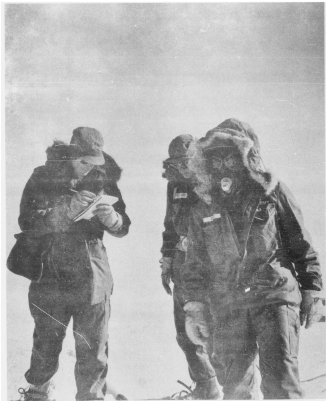
Fig. 6.--Recording air intake as metered at the nozzle of the respirator mask
