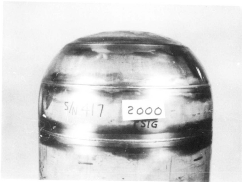
Figure No. 7 - Vessel #417 Stretched at 2000 psi
