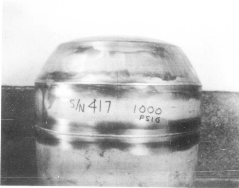
Figure 5 - Vessel #417 Stretched at 1000 psi.
