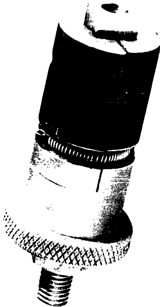
Figure 7. Expansion Plug for Hanging Objects Having Axial Mounting Holes on Three-Wire Pendulum
