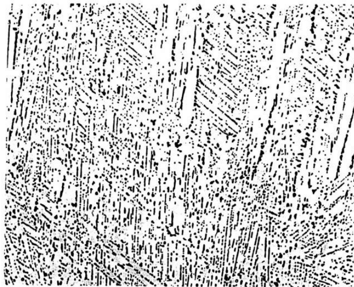
Figure VI:7 - 52 \pm 0.5\% Rh, 6 days, 1320^\circ \pm 20^\circ\text{C} , etchant II. \sigma (dark) + \alpha_1 (white).
