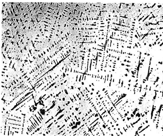
Figure VI:5 - 24 \pm 1\% Rh, as cast, etchant I. \alpha\text{-Ta} (gray) + \sigma (white).
