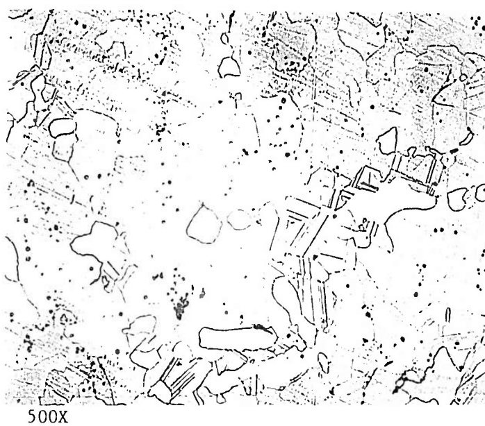
Figure VI:21 - 59.5 \pm 0.5 atomic percent Ir, 17 hours, 1992 \pm 15^\circ\text{C} , etchant II. \alpha_2 (twinned, gray) + \alpha\text{-TaIr}_3 (white).
