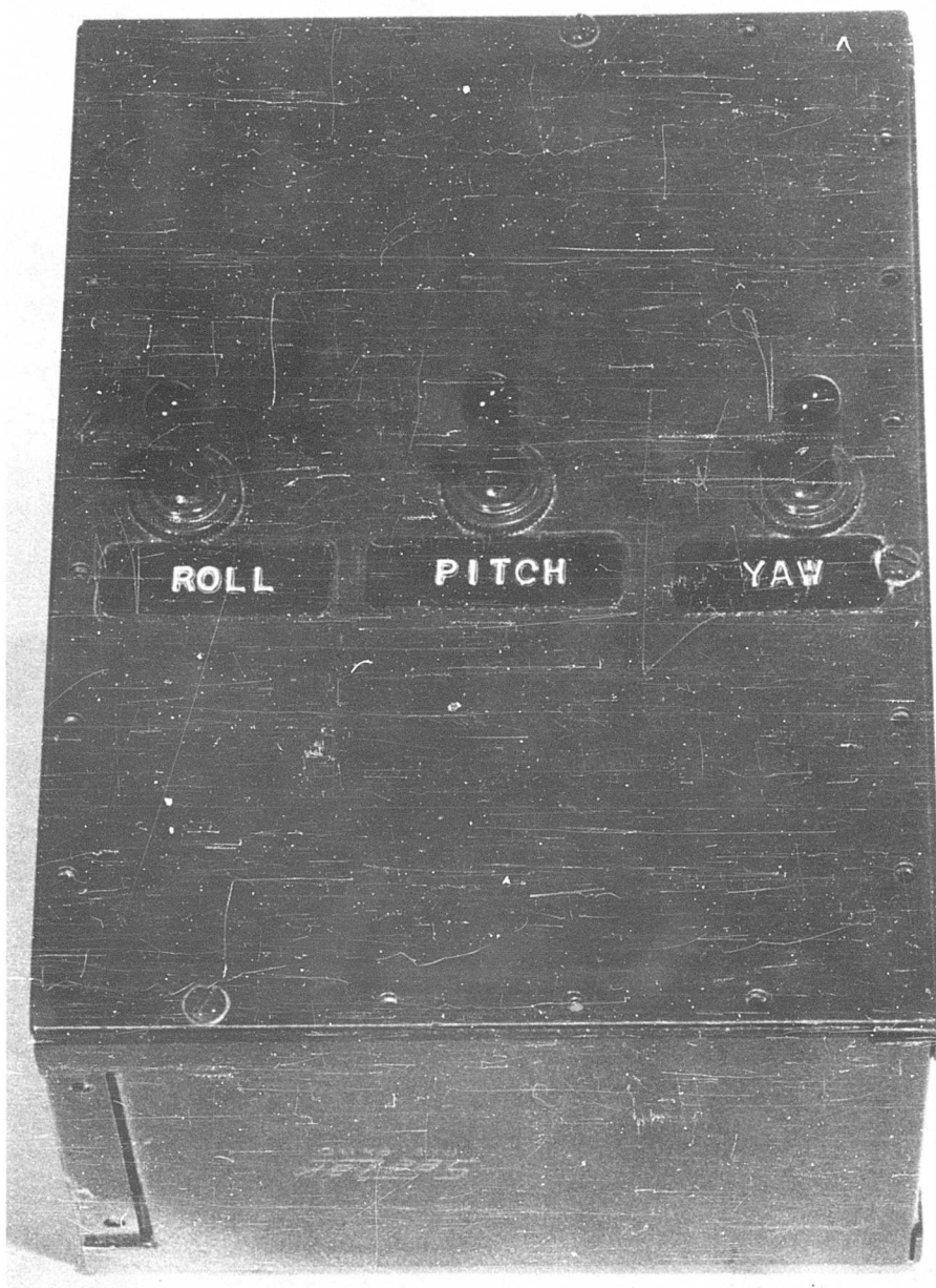
Figure 4. On-Off Toggle Controller
