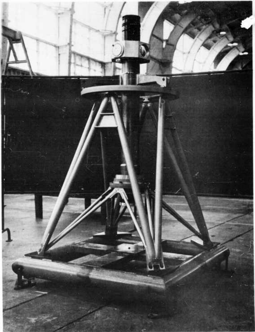
Figure 3.3-1. Initiation of Hub Assembly
