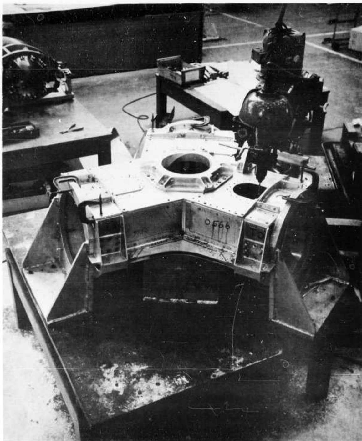
Figure 3.2.2-1. Floating Hub in Process of Assembly
