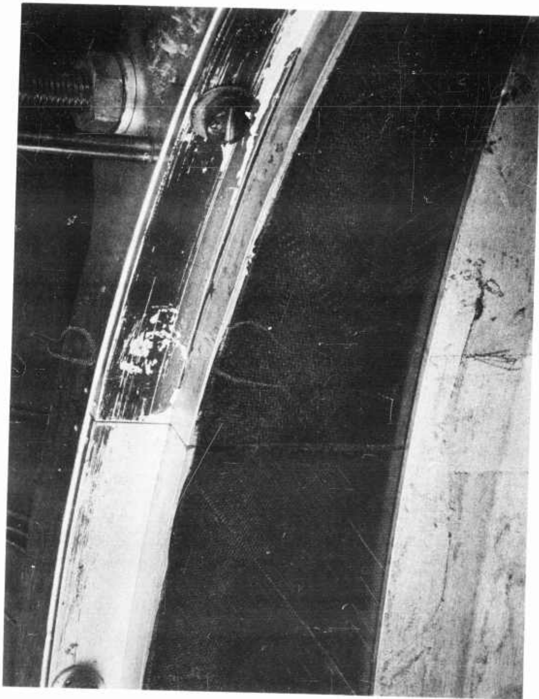
Figure 7-5. Fabroid Bearing after 26.5 hrs. of Test (no apparent damage) Lower Left in Fixture
