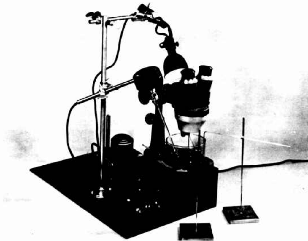
Figure 49 - Electropolishing apparatus used for the preparation of thin specimens for transmission electron microscopy.
