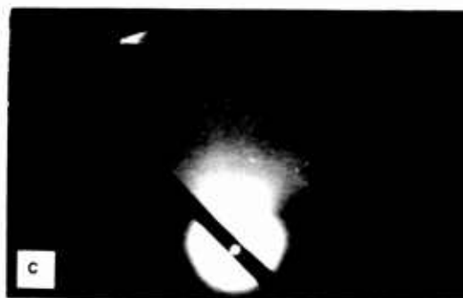
Figure 74 - Electron diffraction photographs of single crystal ground on a (10\bar{1}8) face to remove 2 mils: (a) as-ground; (b) etched 10 sec; (c) etched to remove 1/2 mil. White spot in upper left of each picture is a spurious reflection.
