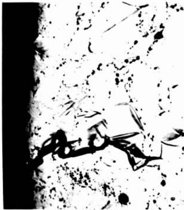
Figure 91 (Cont.) Sequence of deformation and fracture in as-received hot-pressed sheet: (e) advanced stage of fracture (bright light); (f) final fracture. (All photos 500X; polarized light, except (e))
