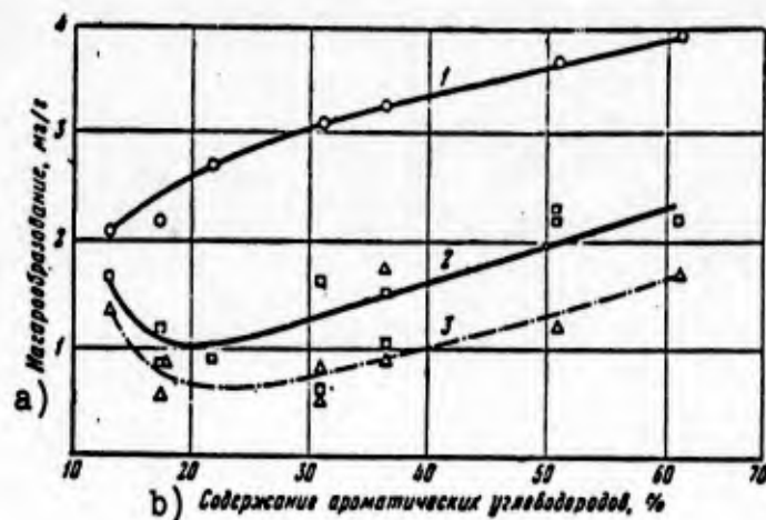
Fig. 94. Variation of scaling as a function of aromatic-hydrocarbon content in fuel and additives to fuel. 1) Without additives; 2) additive A; 3) additive B. а) Scaling, mg/g; б) aromatic-hydrocarbon content, %.
