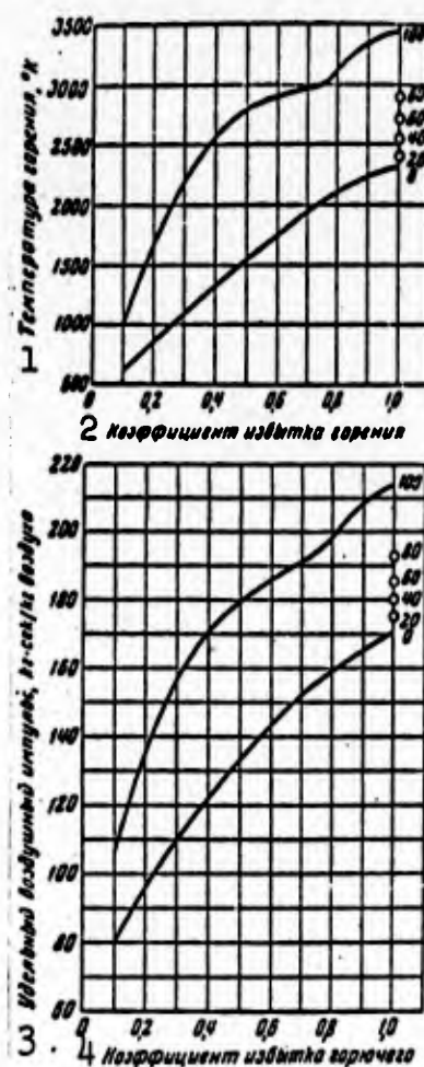
Fig. 65. Theoretical characteristics of the combustion of an aluminum suspension. The figures on the curves indicate the Al content in the octene-1, in % by weight. 1) Temperature of combustion, ^{\circ}\text{K} ; 2) excess combustion [sic - probably combustible] ratio; 3) specific air impulse, \text{kg}\cdot\text{sec}/\text{kg} of air; 4) excess-combustible ratio.
