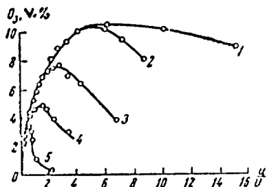
Fig. 1. Dependence of ozone concentration upon the factor \frac{u}{v} for reactor 1: 1) 780 mm Hg; 2) 620 mm Hg; 3) 440 mm Hg; 4) 320 mm Hg; 5) 160 mm Hg.
