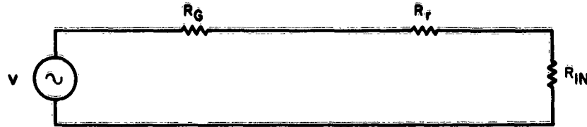
Figure 7. Effective Crystal Circuit in Series Resonant Oscillator
