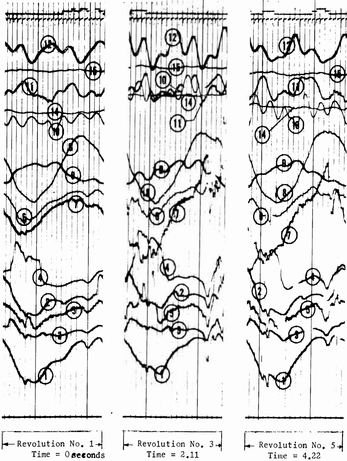
FIGURE 38e - THREE ROTOR REVOLUTIONS OSCILLOGRAPH NO. 5 CONDITION NO. 34, SYMMETRICAL PULL-UP.
