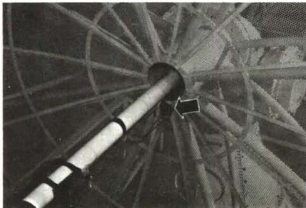
Figure 10. Accelerometer Installation RCA Tx Steerable Antenna Dish.
