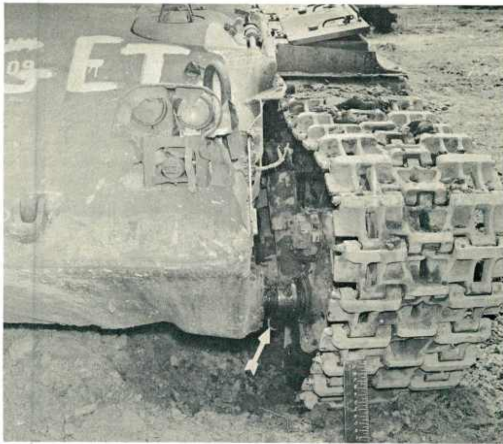
Figure 3 - B30536: Front View of Left Side of U. S. M47 Tank, No. 30164309, After Detonation of Charge No. 2 Under Centerline of No. 1 Road Wheel, Under Lateral Center of the JSIII Track. Charge Consisted of 7.04 Pounds of Comp B Encased in an 8.5-Inch-Diameter, Cylindrical, 24-Gauge, Galvanized Container, Emplaced with 3-Inch Soil Cover.
