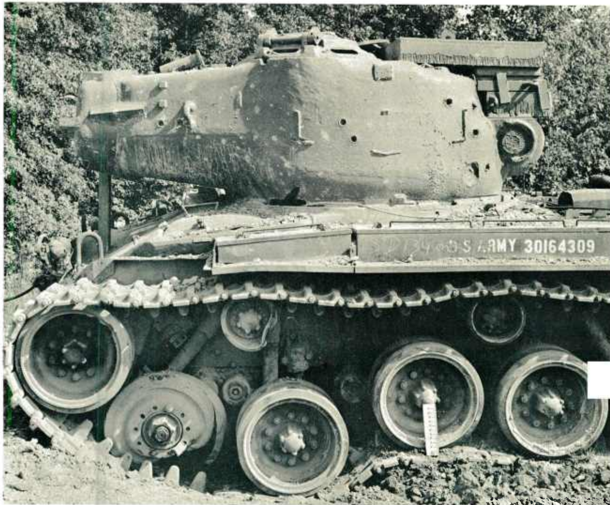
B31646: General View of Left Side of U. S. M47 Tank, No. 30164309 After Detonation of Charge No. 3 Under Centerline of No. 1 Road Wheel Under the Lateral Center of the JSIII Track. Charge Consisted of 8.05 Pounds of Comp B Encased in an 8.5-Inch Diameter Cylindrical 24-Gauge Galvanized Container Emplaced with 3-Inch Soil Cover.
