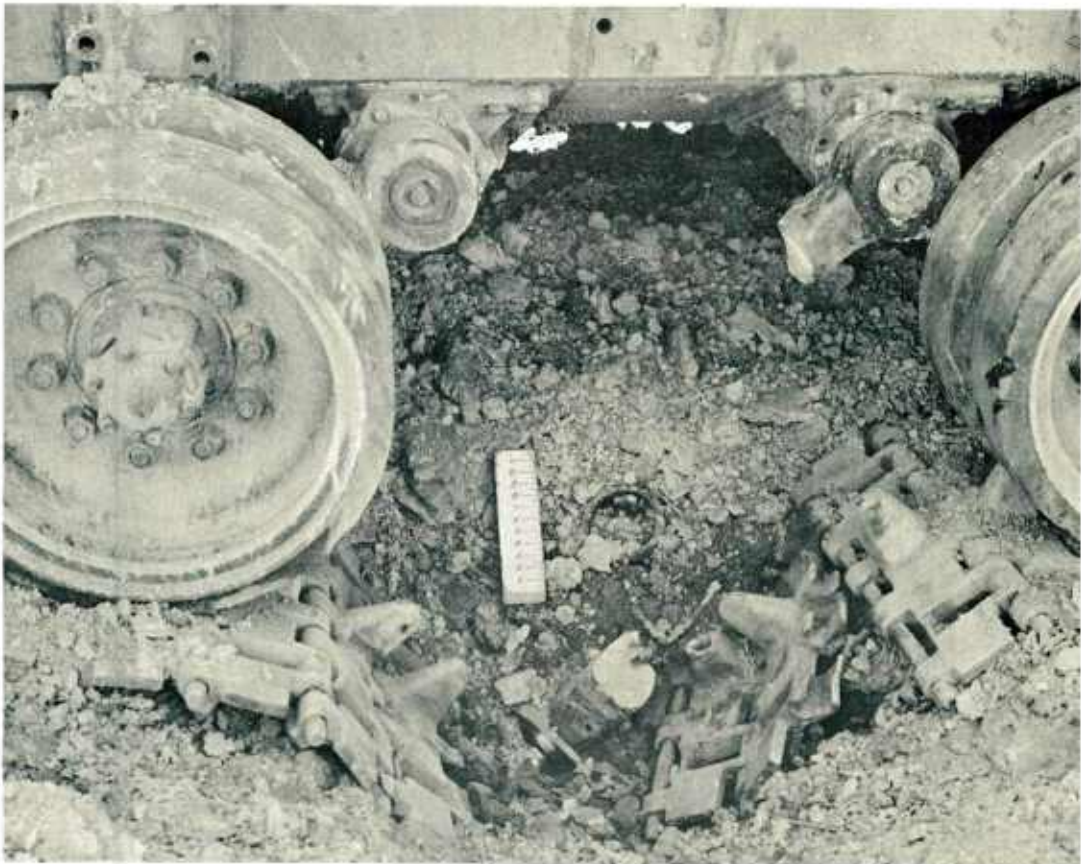
Figure 10 - 59T1854: Closeup of Right Side of U.S. M47 Tank, No. 30164306 After Detonation of Charge No. 22 Under Centerline of No. 3 Road Wheel Under Lateral Center of the JSIII Tank Track. Charge Consisted of 2.98 Pounds of H6 Encased in an 8.5-Inch-Diameter, Cylindrical, 24-Gauge, Galvanized Container. Emplaced with 3-Inch Soil Cover.
