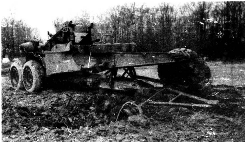
Figure 10 (C): Slight Damage Incurred by other GOER Tire and Test Carriage.
