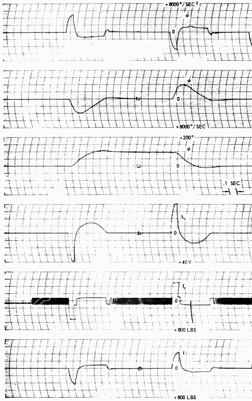
Figure 3.7.66. Transient Responses Mach 5 Altitude 60K \phi_c \pm 90^\circ .
