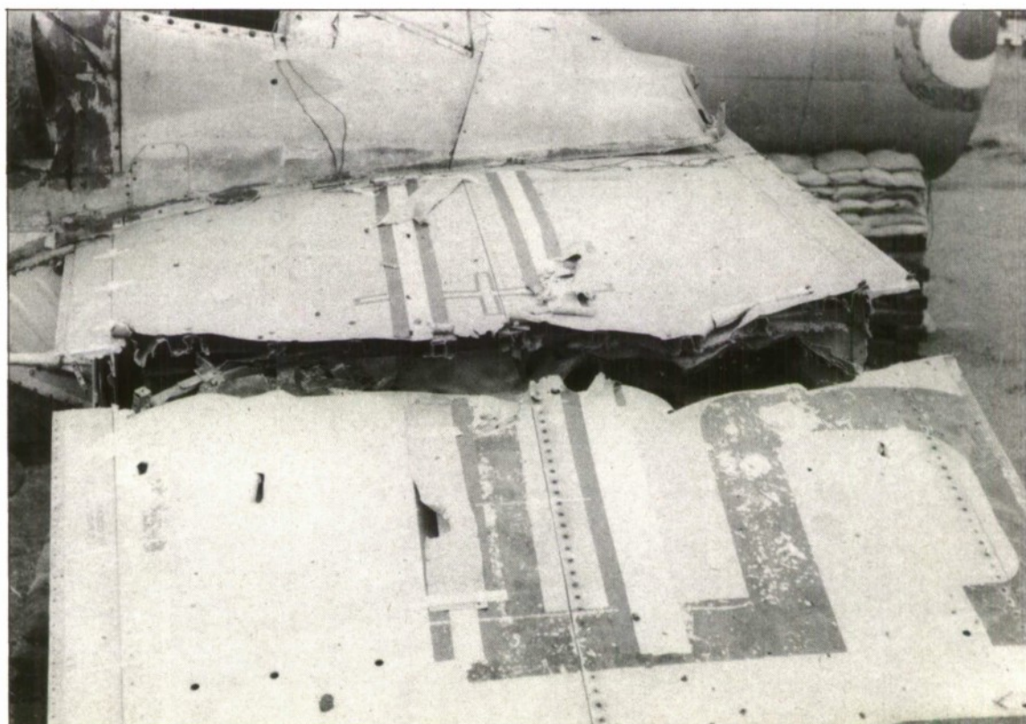
FIG.13b. FIRING 6. DAMAGE TO WING LOWER SURFACE LOOKING INBOARD (1/4 inch ROD, STATION 442)
