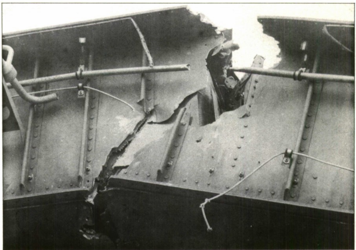
FIG.13c. FIRING 6. SEVERED REAR SPAR (1/4 inch ROD, STATION 442)
