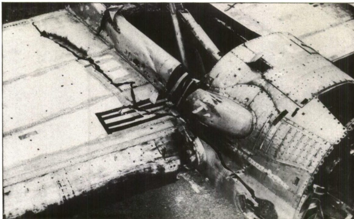
FIG.9a. FIRING 4. ROD DAMAGE TO LOADED PORT WING (1/4 inch ROD, STATION 225, 1½ g FLIGHT LOADS)
