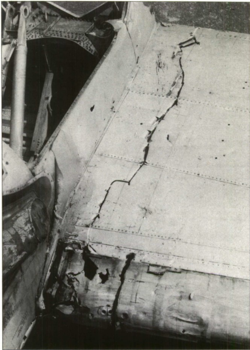
FIG.7a. FIRING 2. ROD DAMAGE TO LOADED STARBOARD WING (3/16 inch ROD, STATION 225)
