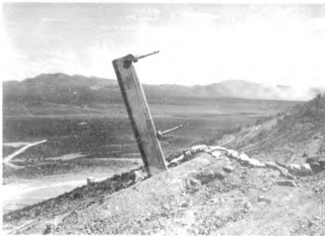
Figure 3.5 Typical gage installation, back slope.
