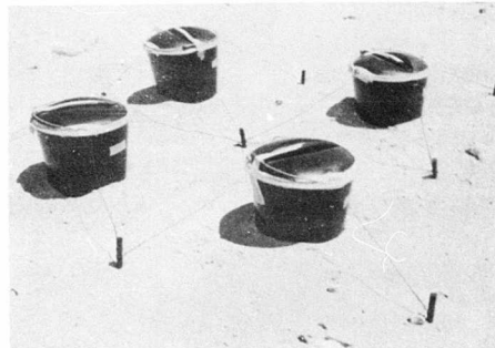
Figure 2.5 Open-type fallout collector installation. (Covers were removed a few hours before the shot.)
