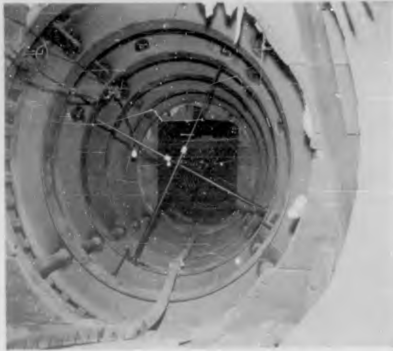
Figure 2.48 Mechanical diameter-change gages installed on wide-flange rings (DASA - NOU 071-06 NTS-62).
