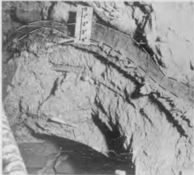
Figure 3.89 West end B3d at 90° (postshot). Note compression of cinders (DASA - NOU 324-04 NTS- 62).
