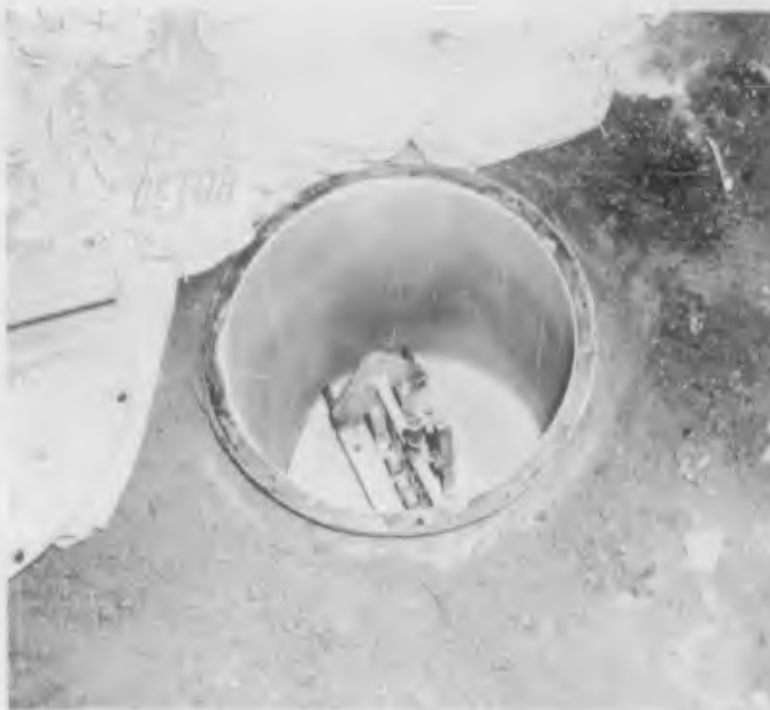
Figure 2.55 Reed gage in canister, oriented to measure radial (horizontal) component of shock (DASA - NOU 083-04 NTS-62).
