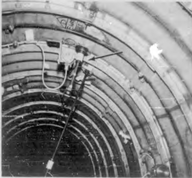
Figure 2.43 Electronic displacement gage installed to measure compression of backpacking material (DASA - NOU 073-10 NTS-62).
