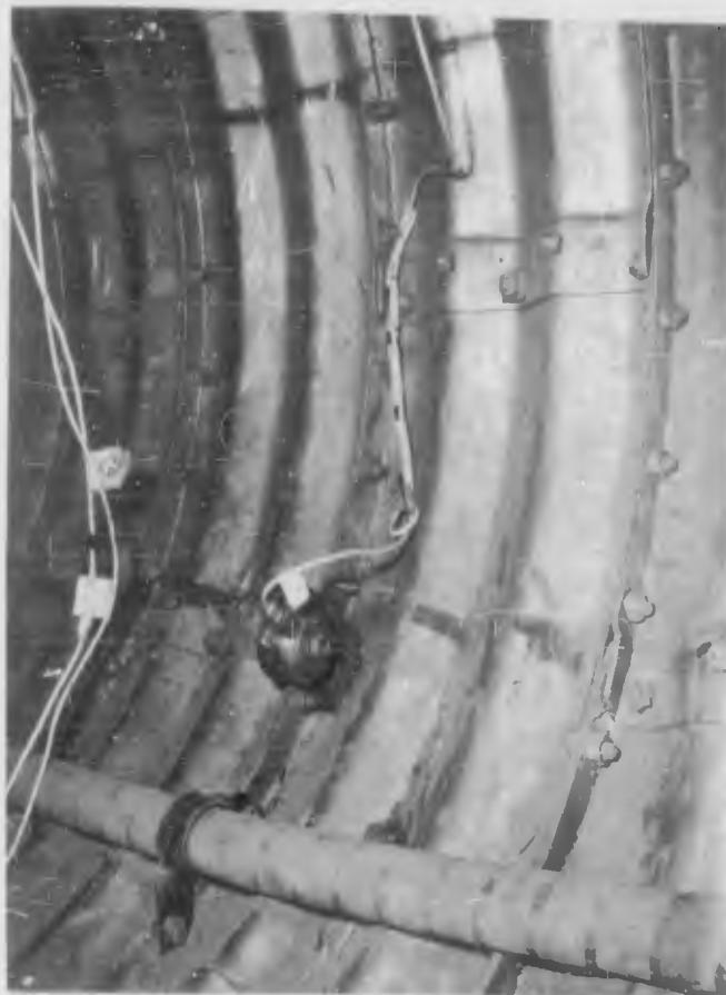
Figure 2.42 Electronic displacement gage mounted to measure diameter change (DASA - NOU 084-05 NTS-62).
