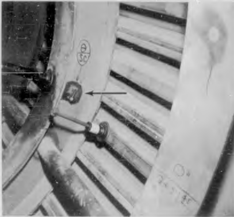
Figure 2.56 DeForest gage installed on wide flange ring to measure circumferential strain (DASA - NOU 071-05 NTS-62).
