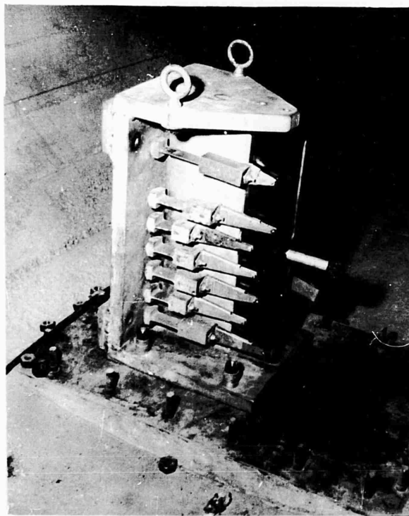
Figure 6 Gage installed vertically in liner structure B3b. (FCWT DASA 043 (NOU-032-05) NTS-62)
