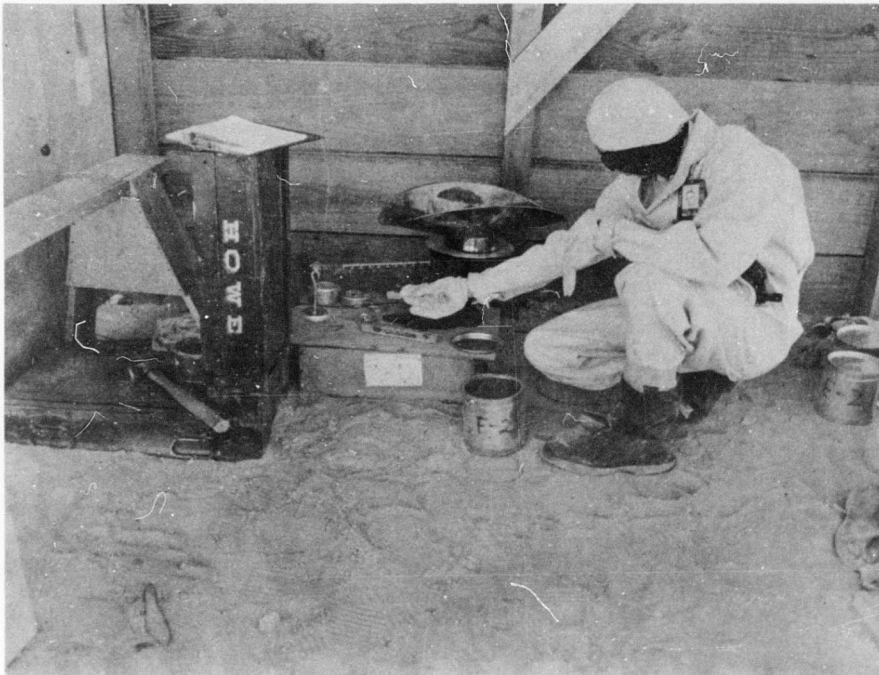
Figure 2.6 Initial weighing and recording of samples. The Howe scale had a 300-pound capacity in 1/4-pound graduations; the Soiltest scale (in use) had a 35-pound capacity in 0.01-pound graduations.
