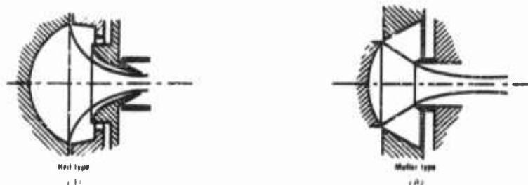
FIGURE 26-7 High-current electron guns
