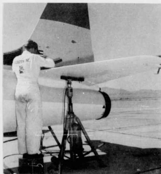
Figure 3.3 Fuselage Calibration. Left, Nose Jacked Up to Prevent Nose Strut Oleo Collapse; Right, Applying Load to Horizontal Stabilizer.
