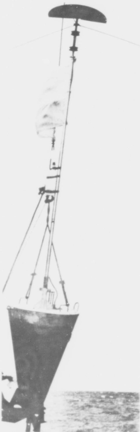
Fig. 3.4 Free-floating Sea Station Being Launched
