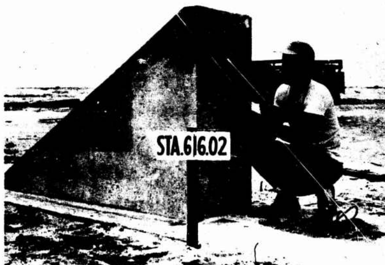
Fig. 4—After-wind (Wiancko) gauge mounted in concrete wedge.
