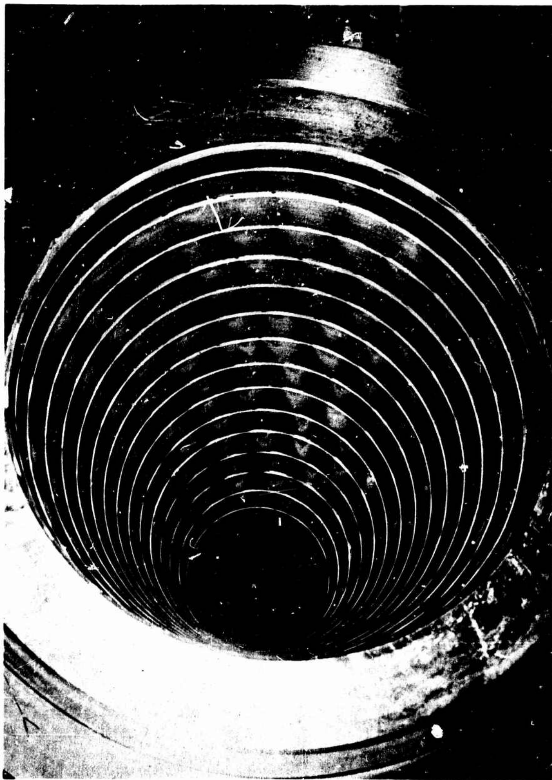
Front View, Cooled Throat after Nine Tests
