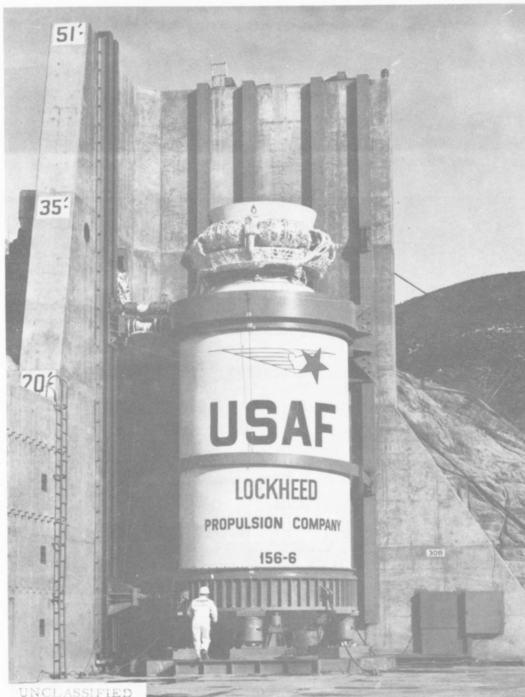
Figure 10 Completely Assembled Motor 156-6 in Test Stand
