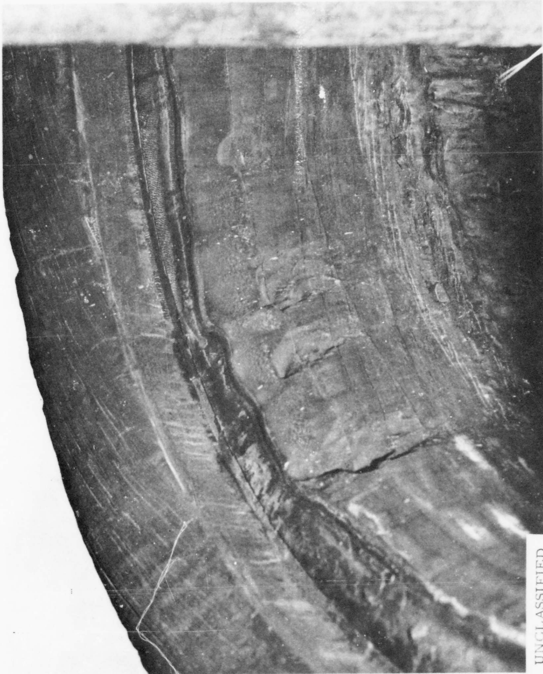
Figure 47 Postfire View of Entrance Cap and Throat Section
