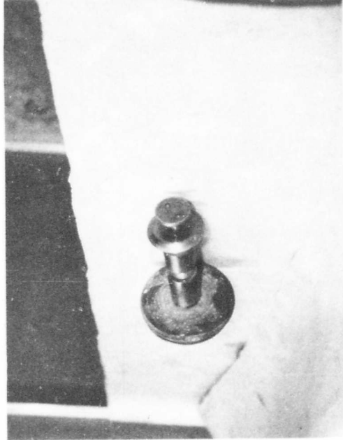
d. Pintle Structure - Postfire
