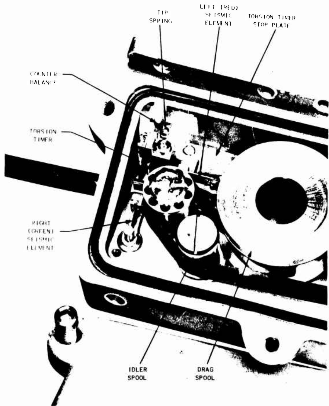
Fig. A.47 Accelerometer, Self-recording Type, with Main Cover Removed Showing Tape in Place Ready for Recording
