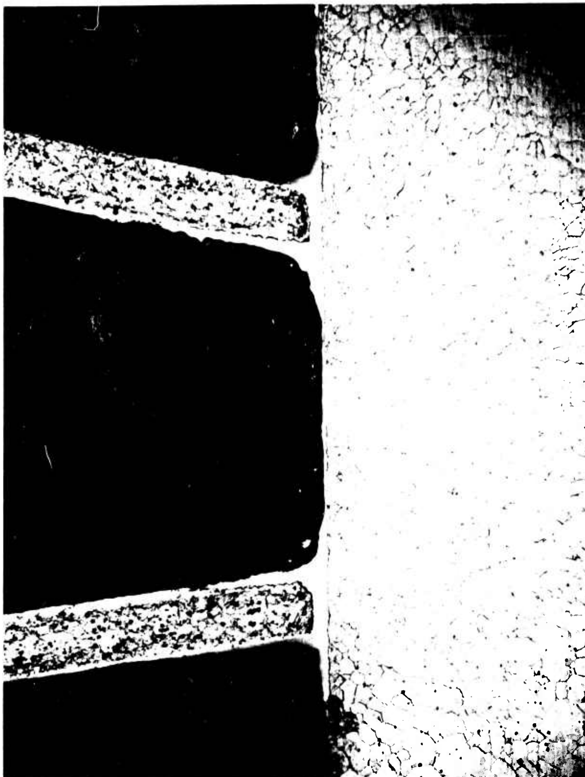
Figure 113. Face Sheet to Honeycomb Braze
