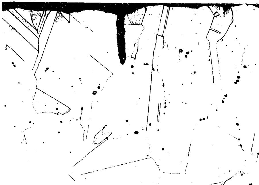
Figure 24. High Magnification Photomicrograph of Section Showing Gassing (Spherical Voids)
