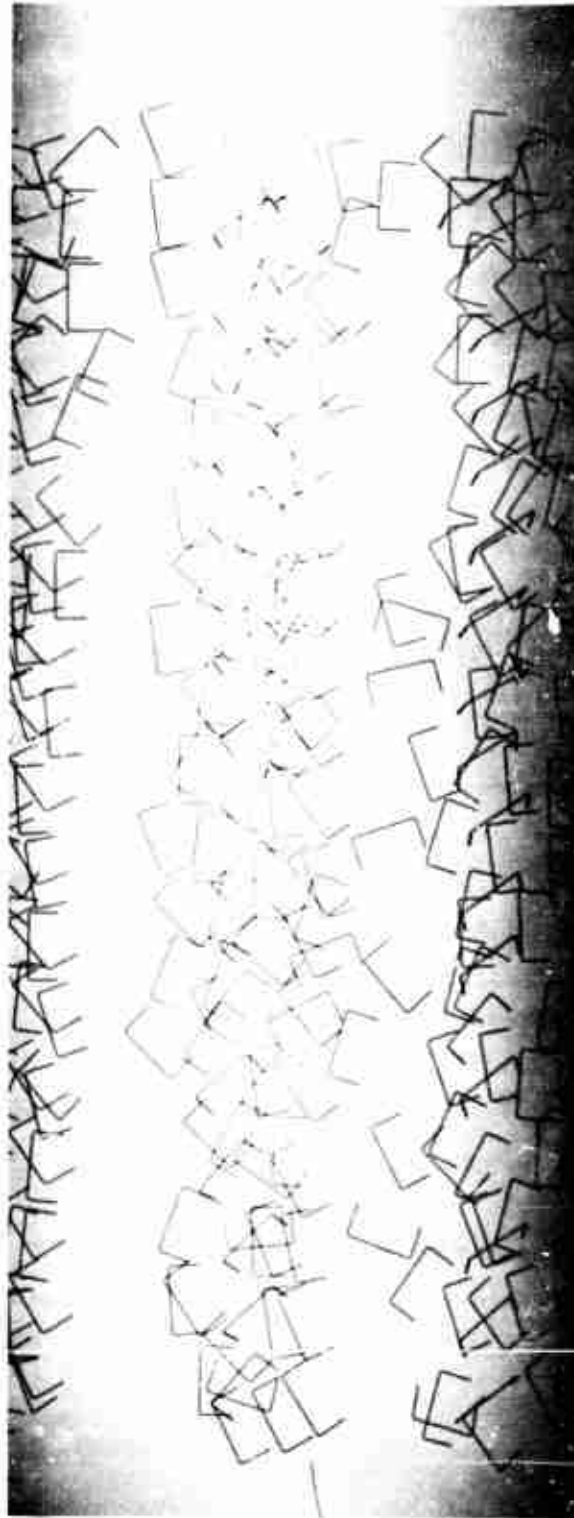
Figure 6. X-Ray of Radial Staple Reinforced Grain (Diametric view shows staples aligned in circumferential plane)
