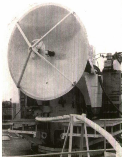
The 6 ft. diameter aerial.
