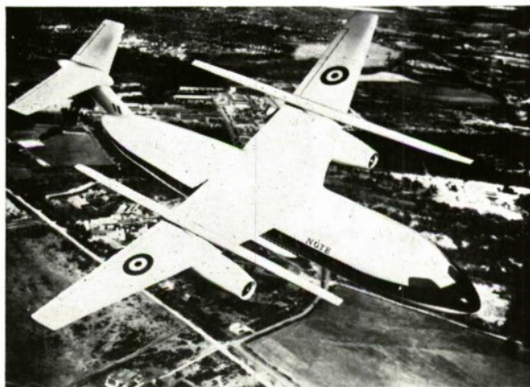
FIG. 1. A glimpse of the future?—Low noise level vertical take-off and descent combined with high speed cruise using N.G.T.E. circulation-controlled stoppable rotors.
