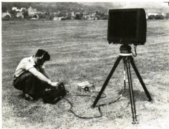
Portable radar for detection of movement in clutter. It uses pulse doppler techniques with visual and aural presentation.
