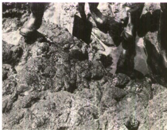
FIG. 2. Oil and sand mixture with a consistency of clay.
