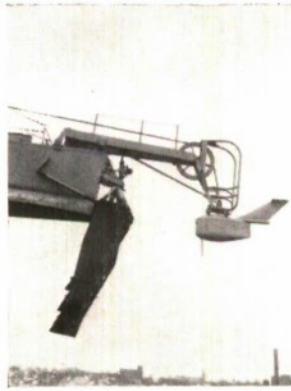
FIG. 6. Hydrofoil craft "Baddeck" (formerly "Bras D'Or") fitted for towing, with experimental towed body shown at right.
