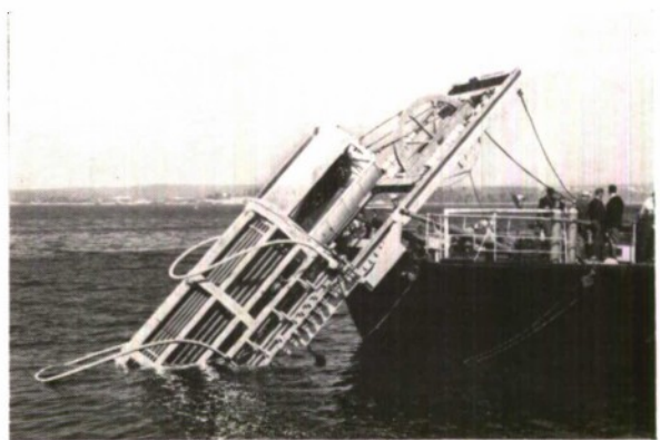
FIG. 4. Pod with explosive charges and trainable hydrophone array being lowered over the stern of CNAV "Fort Frances".
