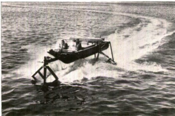
FIG. 7. Experimental hydrofoil craft Rx.
