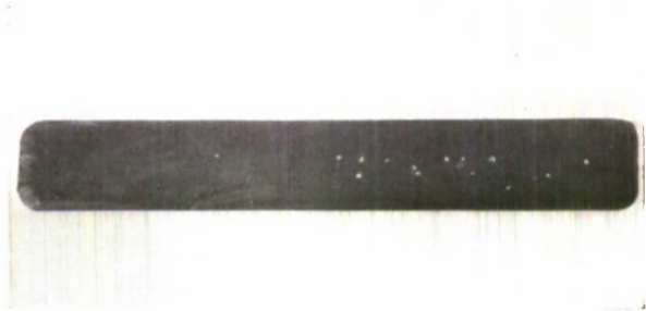
FIG. 13. Porosity and undercure.
