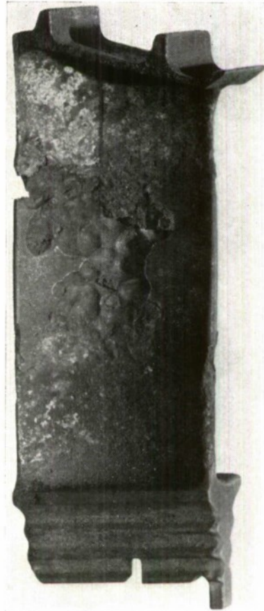
FIG. 2. Corroded turbine blade
