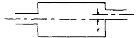
(b.) OUTLET PLACED FOR MODE SUPPRESSION
