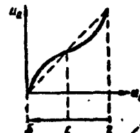
Fig.5. Amplitude characteristic of gamma-corrector
