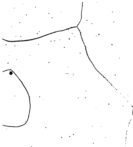
Fig. 4 - High-purity iron vacuum-annealed for 1 hr at 1800°F, then furnace cooled; electropolished (200X)
