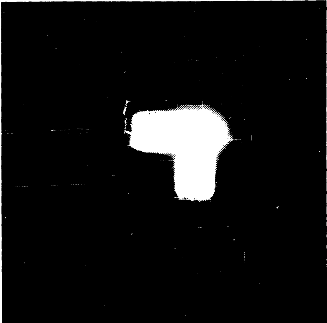
Figure 17 - Intersection of Two 7-mc. Shear Wave Packets in a Glass Specimen
