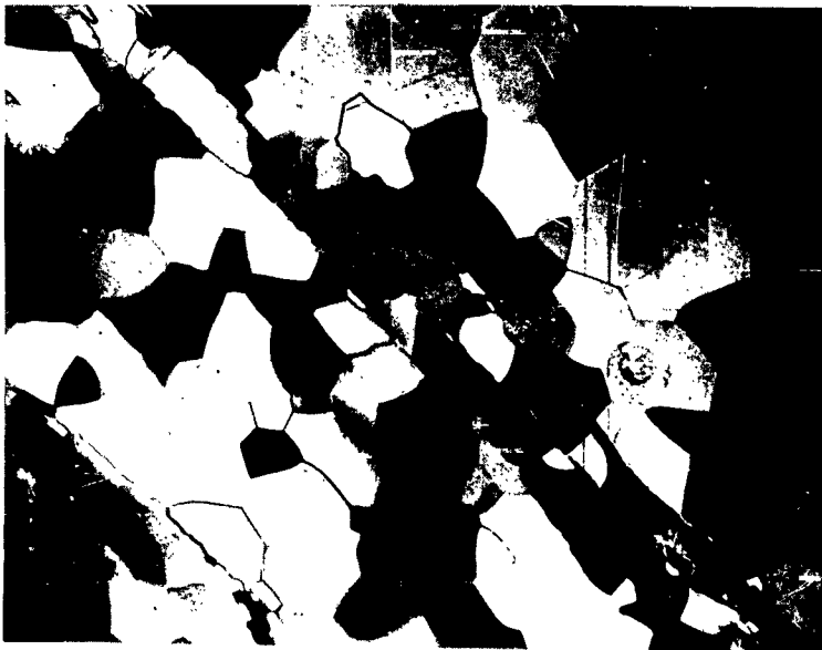
FIG. 9. S-7 ANNEALED AT 700°C FOR 20 MINUTES. LONGITUDINAL SECTION. POLARIZED LIGHT, 100X.
