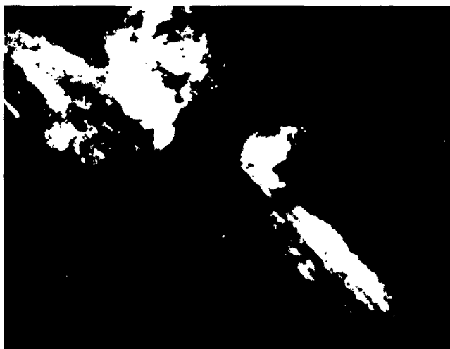
(b) Weak Silver- \text{Al}_2\text{O}_3 (Whisker) Composite Showing 'Pull-out' at the Fracture. Whiskers Were Not Metallized (70X)
